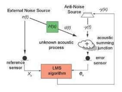
Closed-loop control diagram.
