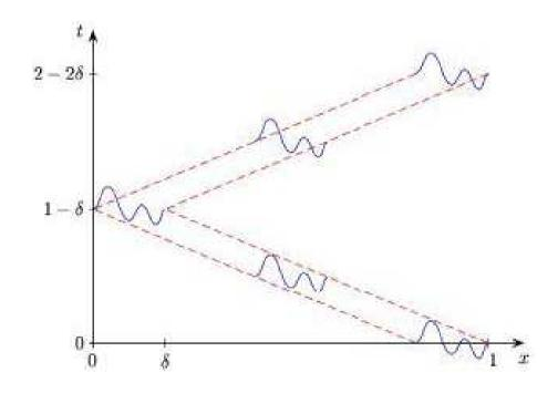
Wave localized at t=0 near the extreme x=1 that propagates with velocity one to the left, bounces on the boundary point x=0 and reaches the point of observation x=1 in a time of the order 2.
