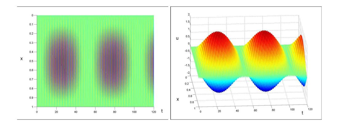
$h=1/61,\ N=60,\ 0\leq t\leq 120.$  The solution exhibits a time-periodicity property with period  $\tau$  of the order of  $\tau\sim 50$  which contradicts the time-periodicity of period 2 of the wave equation. High frequency wave packets travel at a group velocity  $\sim h$ .
