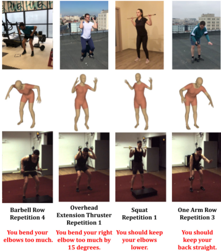
Figure 5.1: Textual and visual feedback produced by our AIFit on real world videos, captured with a regular smartphone camera. We use MubyNet-FT to estimate the 3d pose of the trainee. For each example, we show the following: an image with the identified error of the trainee ( top row ), the 3d reconstruction of the trainee ( second row ), the corresponding image with the correct execution of the instructor ( third row ) and the textual feedback ( bottom row ). The two examples on the ( left ) show active features feedback, while the two on the ( right ) show passive features feedback. Notice generalization to various humans in different environments and camera viewpoints.
