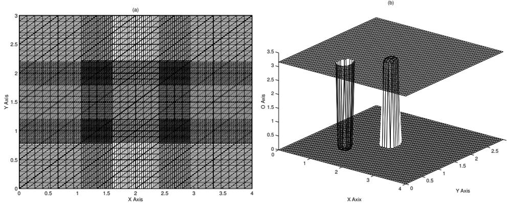
Figure 1: (a) Meshes  $\mathcal{T}_H$ ,  $\mathcal{T}_h$ , and the domain decomposition, (b) Obstacles  $a$  and  $b$ .
