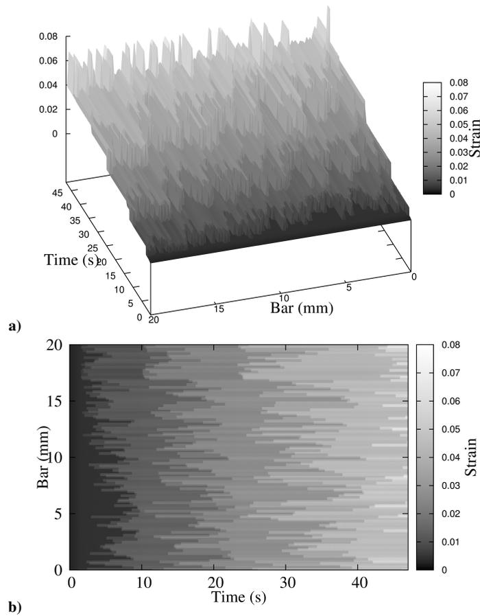
**Fig. 7.9** Overall picture of the strain evolution in the bar during the cross-head velocity controlled experiment in Fig. 7.6. **a)** Spatial representation of  $\epsilon = \epsilon(X, t)$ . **b)** Its plane projection
