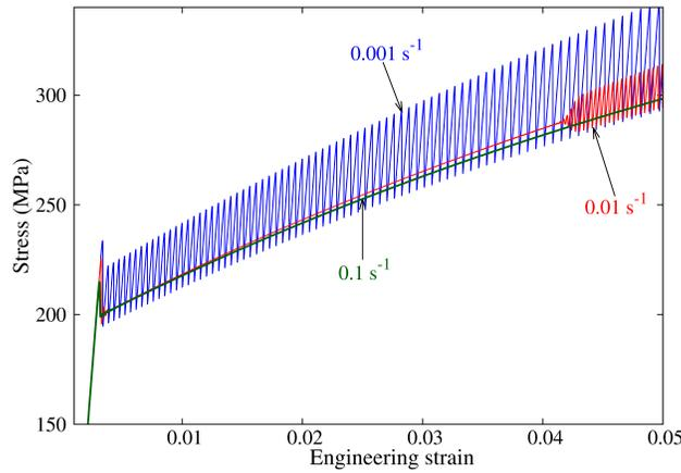
**Fig. 7.24** Elastic-viscoplastic homogeneous process with strain hardening described by the non-autonomous system (7.47) for three imposed engineering strain-rates:  $\dot{\varepsilon}_e = 10^{-3} \text{ s}^{-1}$ ,  $\dot{\varepsilon}_e = 10^{-2} \text{ s}^{-1}$  and  $\dot{\varepsilon}_e = 10^{-1} \text{ s}^{-1}$  when  $\dot{\varepsilon}_0 = 3.5 \times 10^{-6} \text{ s}^{-1}$  ( $\tau = 2.85 \times 10^5 \text{ s}$ )
