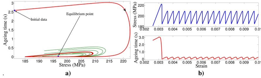
**Fig. 7.21 Unstable Focus Interval:**  $\dot{\epsilon}_e = 10^{-3} \text{ s}^{-1}$  and  $\dot{\epsilon}_0^* = 3.5 \times 10^{-6} \text{ s}^{-1}$  ( $\tau^* = 2.85 \times 10^5 \text{ s}$ ). Homogeneous process described by (7.50) **a)** Phase portrait. **b)** Stress and ageing time vs. strain
