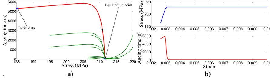
**Fig. 7.19 Stable Node Interval:**  $\dot{\epsilon}_e = 5 \times 10^{-7} \text{ s}^{-1}$  and  $\dot{\epsilon}_0^* = 3.5 \times 10^{-6} \text{ s}^{-1}$  ( $\tau^* = 2.85 \times 10^5 \text{ s}$ ). Homogeneous process described by (7.50) **a**) Phase portrait **b**) Stress and ageing time vs. strain
