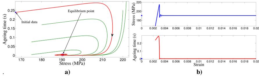
**Fig. 7.22 Stable Focus Interval:**  $\dot{\epsilon}_e = 10^{-2} \text{ s}^{-1}$  and  $\dot{\epsilon}_0^* = 3.5 \times 10^{-6} \text{ s}^{-1}$  ( $\tau^* = 2.85 \times 10^5 \text{ s}$ ). Homogeneous process described by (7.50) **a)** Phase portrait. **b)** Stress and ageing time vs. strain
