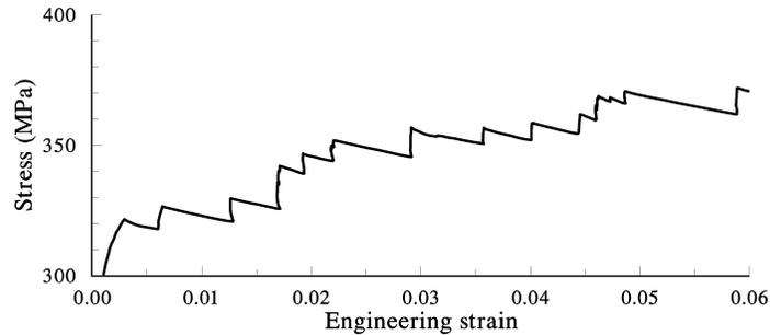
**Fig. 7.5** Strain bursts in a Zwick testing machine in a nearly constant stress-rate test  $\dot{\sigma} \approx 0.076 \text{ MPa/s}$  for a 5182H28 alloy (reproduced with permission from Făciu et al. [Făc1998] ©EDP Sciences)
