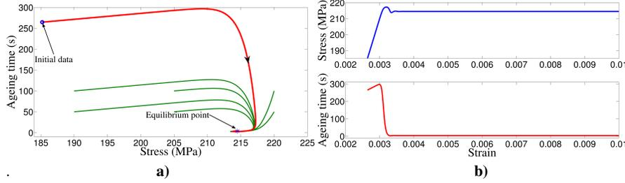
**Fig. 7.20 Stable Focus Interval:**  $\dot{\epsilon}_e = 10^{-5} \text{ s}^{-1}$  and  $\dot{\epsilon}_0^* = 3.5 \times 10^{-6} \text{ s}^{-1}$  ( $\tau^* = 2.85 \times 10^5 \text{ s}$ ). Homogeneous process described by (7.50) **a**) Phase portrait **b**) Stress and ageing time vs. strain
