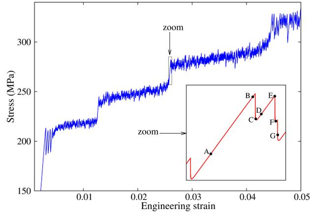
**Fig. 7.6** Serrated stress-strain curve for numerical simulation of a hard-testing machine experiment with engineering strain-rate  $\dot{\epsilon}_e = 10^{-3} \text{ s}^{-1}$ . Insert: zoom of a portion and the position of points A, B, C, D, E, F, G where are recorded the distribution of strain  $\epsilon$  and strain-rate  $\dot{\epsilon}$  in bar, illustrated in Fig. 7.8
