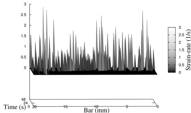
**Fig. 7.10** Overall picture of the strain-rate  $\dot{\epsilon} = \dot{\epsilon}(X, t)$  in the bar during the cross-head velocity controlled experiment in Fig. 7.6
