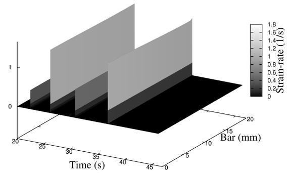
**Fig. 7.17** Overall picture of the ageing time  $t_a = t_a(X, t)$  in the bar during the true constant stress-rate experiment ( $\beta = 1$ ) in Fig. 7.14
