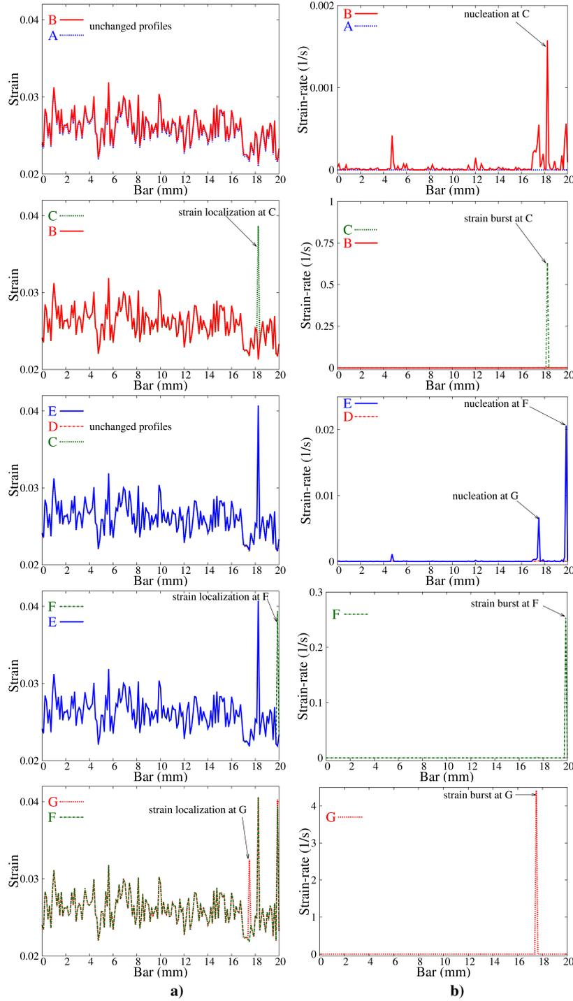
**Fig. 7.8** The distribution of strain  $\epsilon$  and strain-rate  $\dot{\epsilon}$  in bar at the moments A, B, C, D, E, F, G in Fig. 7.6. Note the different scales used for the strain-rate distribution
