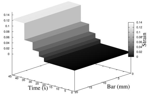
**Fig. 7.16** Overall picture of the strain-rate  $\dot{\varepsilon} = \dot{\varepsilon}(X, t)$  in the bar during the true constant stress-rate experiment ( $\beta = 1$ ) in Fig. 7.14
