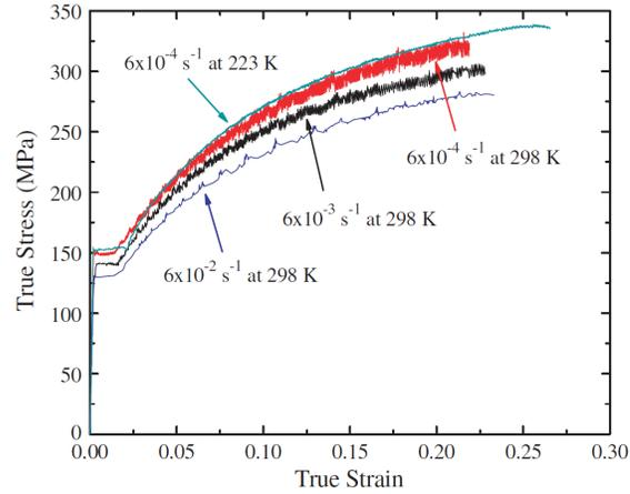
**Fig. 7.1** True stress-strain curves of AA5754 alloy at various strain-rates and temperatures (reproduced with permission from Halim et al. [Hal2007] ©Elsevier Ltd.)
