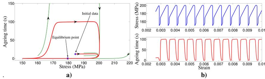
**Fig. 7.23 Unstable Node Area:**  $\dot{\epsilon}_e = 2.2 \times 10^{-4} \text{ s}^{-1}$  and  $\dot{\epsilon}_0 = 6. \text{ s}^{-1}$  ( $\tau = 0.16 \text{ s}$ ). Homogeneous process described by (7.50) **a)** Phase portrait. **b)** Stress and ageing time vs. strain
