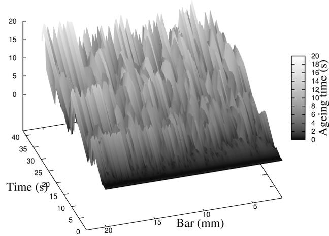
**Fig. 7.11** Overall picture of the evolution of the ageing time  $t_a = t_a(X, t)$  in the bar during the cross-head velocity controlled experiment in Fig. 7.6
