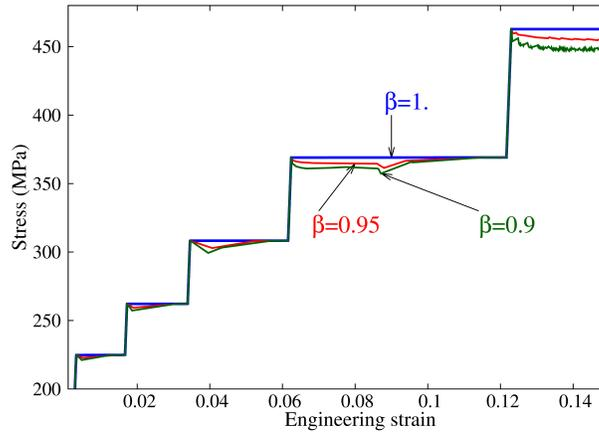
**Fig. 7.14** Staircase type stress-strain curves in the numerical simulation of a soft-testing machine experiment.  $\beta = 1$  corresponds to a true constant stress-rate test (7.43) at  $\dot{\sigma}_e = 10$  MPa/s.  $\beta = 0.95$  and  $\beta = 0.9$  correspond to the mixed boundary condition (7.44) where  $\dot{\sigma}_e = 10$  MPa/s and  $V^* = 2.85 \times 10^{-3}$  mm/s ( $\dot{\varepsilon}_e = 1.4 \times 10^{-3}$  s $^{-1}$ , i.e.  $\dot{\sigma}_e = E\dot{\varepsilon}_e$ )
