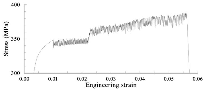
**Fig. 7.7** Nominal stress vs. engineering strain in constant strain-rate test at  $\dot{\epsilon}_e = 10^{-5} \text{ s}^{-1}$  in 5182H28 alloy. Serrated flow with change of plateaus (reproduced with permission from [Făciu et al. [Făc1998] ©EDP Sciences)
