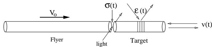
Figure 7: Longitudinal impact of thin bars
